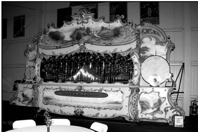
Figure 12. The Wurlitzer Style 180 band organ. 510 pipes and a large scale roll provide complex music.
