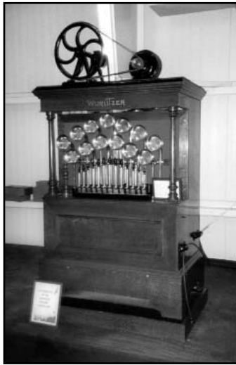
Figure 6 (above). The Wurlitzer Style 105 military band organ with flywheel and motor mounted on top.
