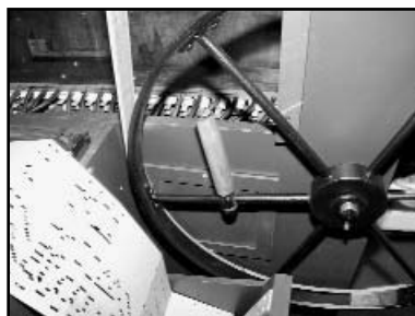
Figure 31 (above). While operating with a motor-driven belt the flywheel retains it's hand-cranked handle.
